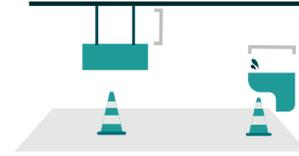
Any objects hanging from the ceiling or protruding **MORE THAN 4"** from the wall must be marked with a cone to be cane detectable.
